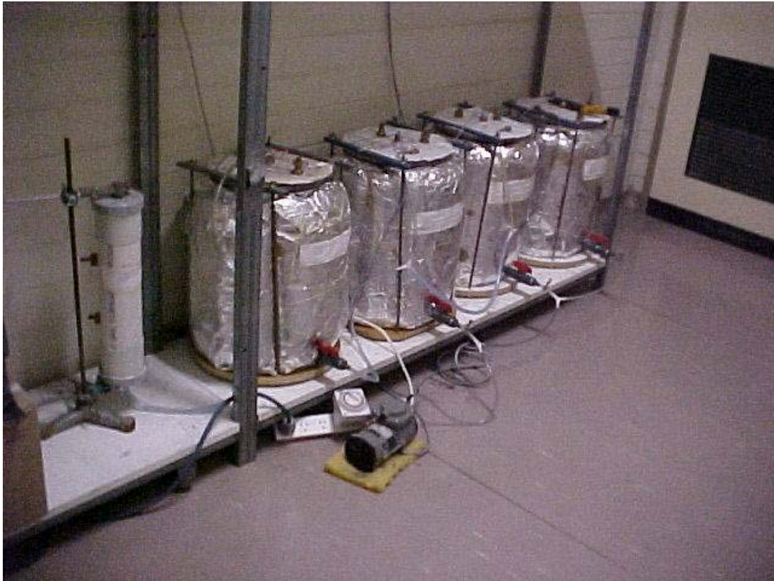
Composters hooked up to an air blower which is controlled by a timer.
