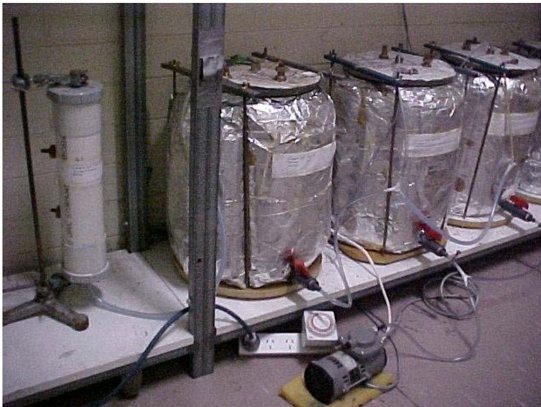
Gases from the composters during aeration are forced through a biofilter and then activated carbon (on far left). No odour can be detected.
