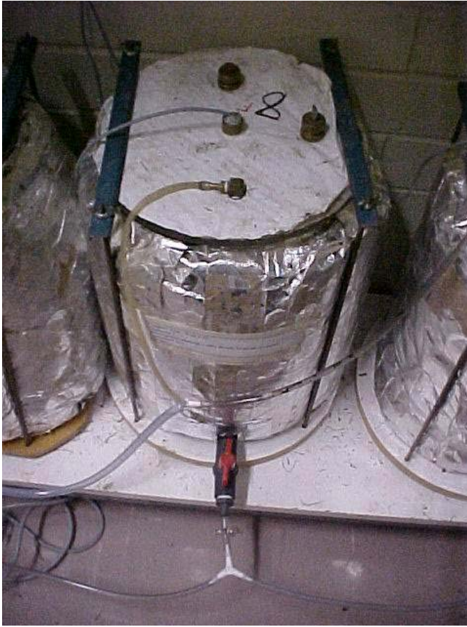
Air enters the bottom of the compostor via a perforated loop embedded in woodchips. Temperature probes are located in the solid matrix.
