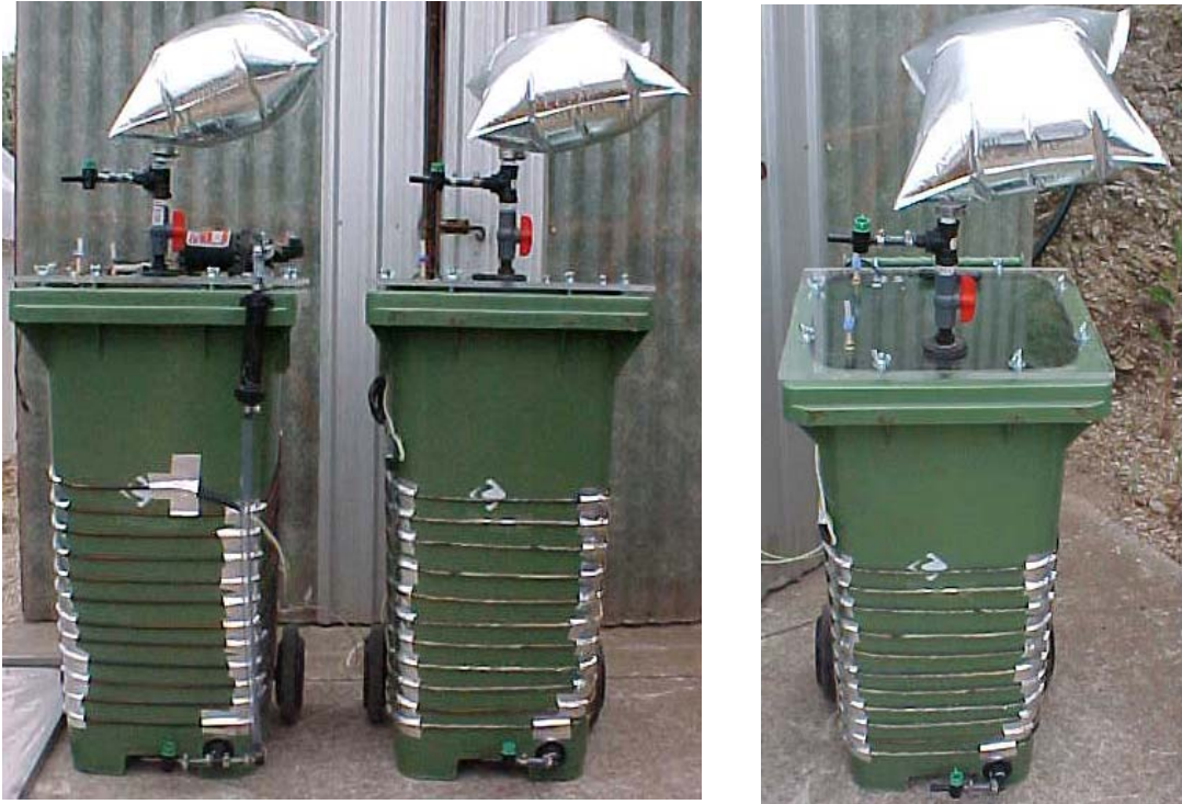
Modified 120L wheelie bin reactors without insulation. Reactor on far left has a pumping recirculation system.
