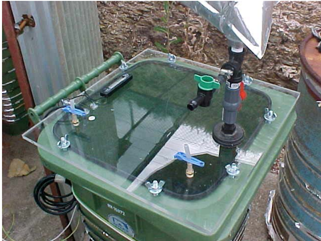
Top of the reactors showing gas sampling ports (blue clips), biogas collection bag and biogas evacuation tap (green tap).
