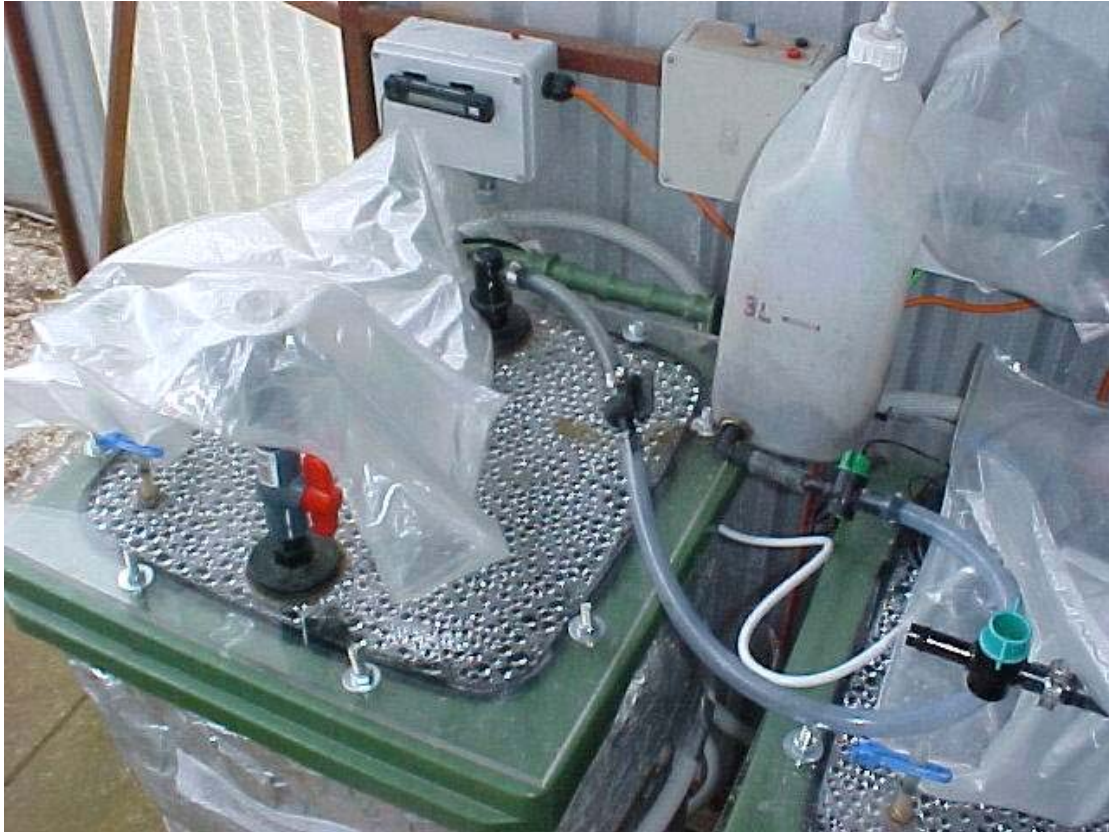
Collected leachate is fed via a tap on the top of the reactor and distributed evenly throughout the system via an irrigation loop.
