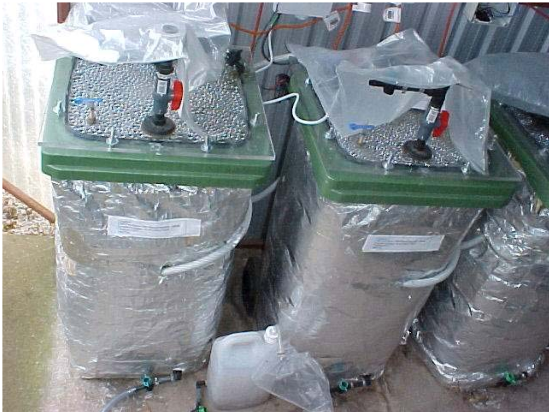
Reactors covered in insulation and heated to 37°C. Leachate is collected via the sample tap to be exchanged with other reactors.
