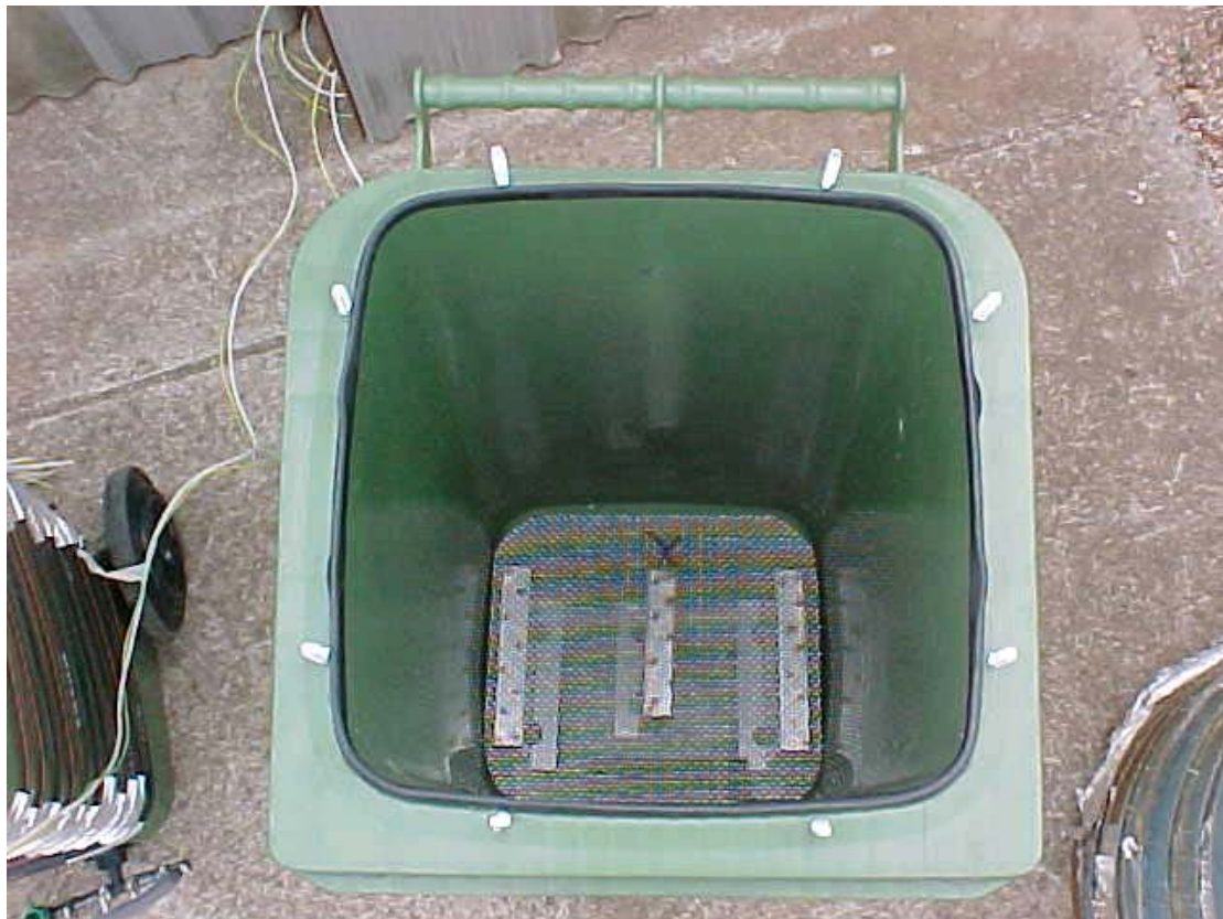
In side the reactor showing 5mm stainless steel sieve used to restrict gross solids entering the leachate sample tap.
