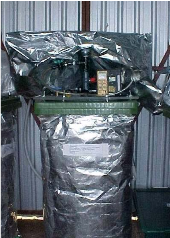
Gas pumps are used to evacuate the gas collection bags via the green biogas taps to determine biogas volume.
