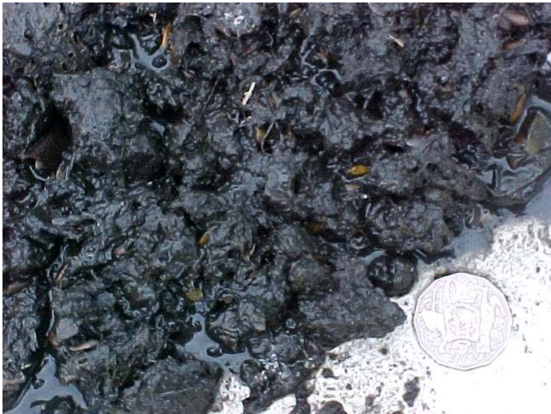
The end anaerobic product after approximately 10 weeks digestion, characterised by small particle size.
