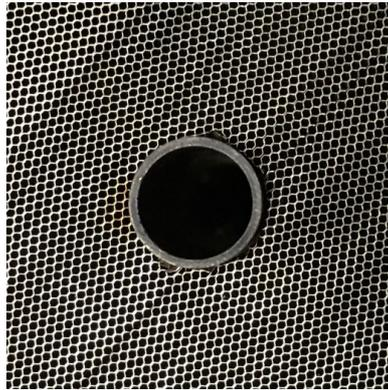
**Figure 1.** Top view of the burner surface.
