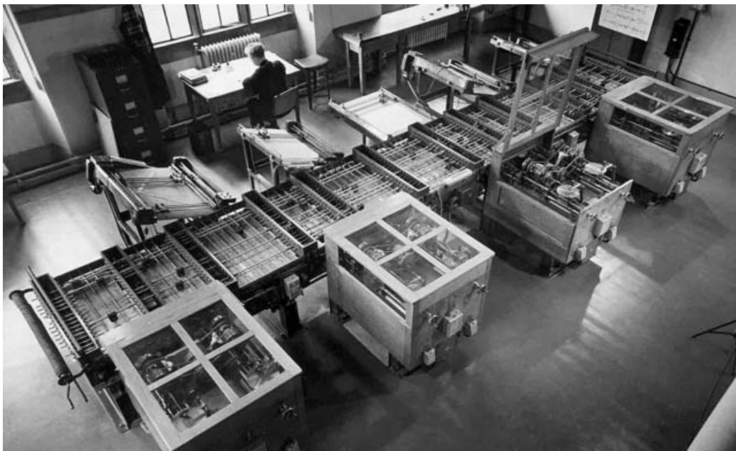
Figure 2: The Cambridge Differential Analyzer, which is similar to Bush's design. The disk-and-wheel integrators are on the right; the input and output tables on the left.
