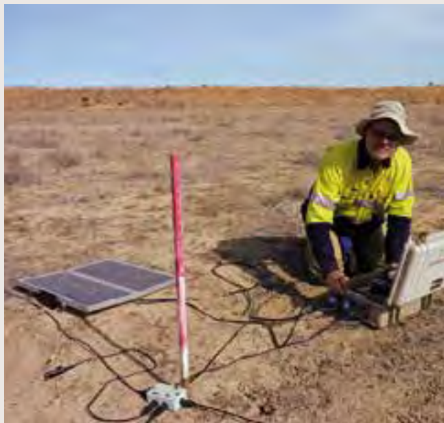
The Electrical Earth Imaging team deploying magnetotelluric equipment in the Cooper Basin.
