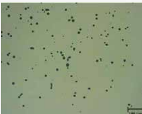
Particles suspended in injected fluid. Left photo (100 µm scale) – low-salinity suspension. Right photo (200 µm scale) – high-salinity suspension.
