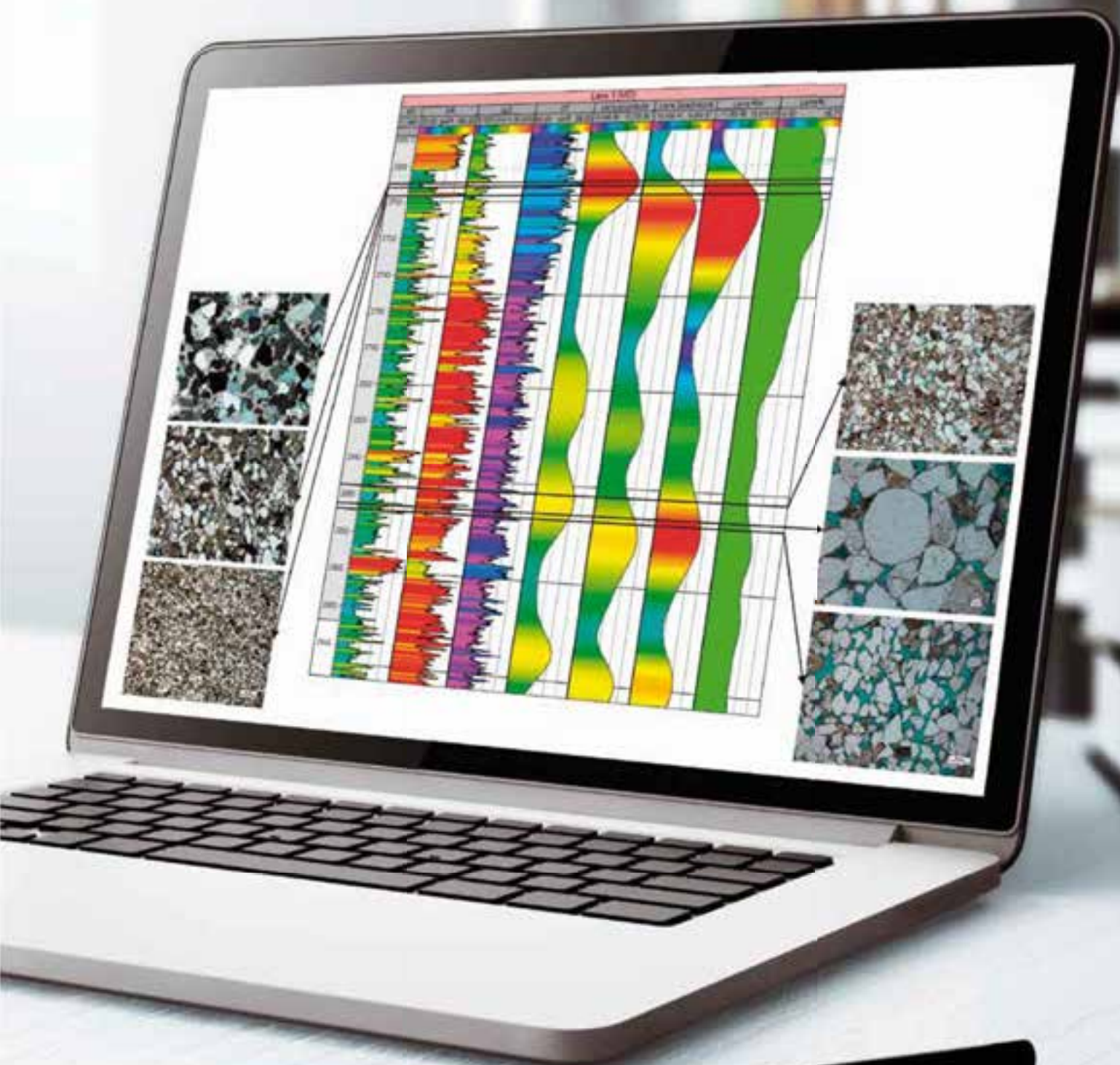
Columnar section of Laira 1, GR: gamma ray, LLD: deep lateral log, DT: sonic velocity, note the higher amplitude and attribute values at 2686 m compared with 1864 m due to porosity variation.
