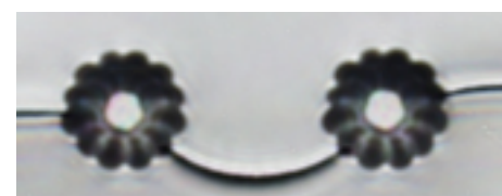
Waveguide written in ZBLAN glass in collaboration with MQ Photonics
