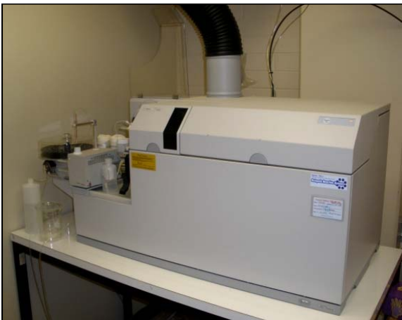
Agilent 7500cs instrument set up for solution mode at Adelaide Microscopy
