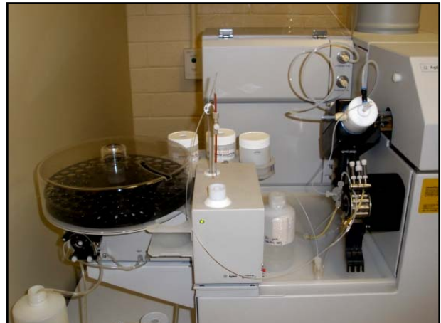
Sample introduction end of the 7500cs
