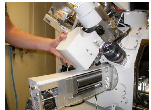
Fitting the analytical accessories - EBSD Spectrometer.
