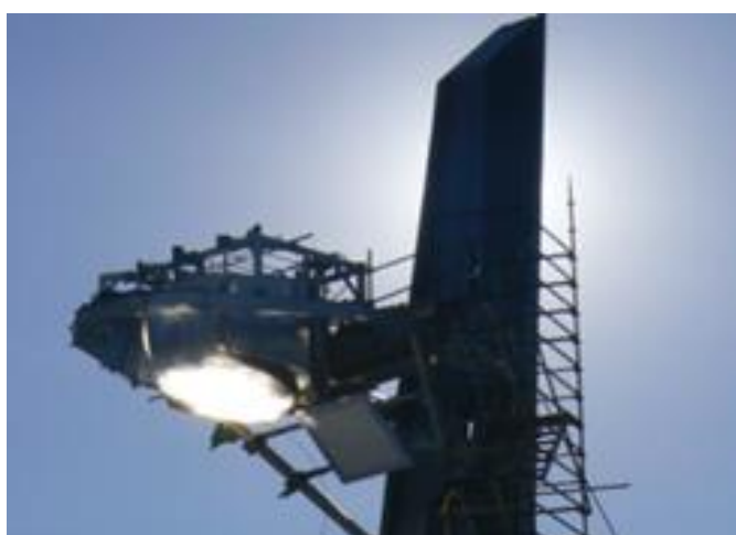
Figure 4: Pilot-scale demonstration of CSIRO's solar steam reforming of natural gas to upgrade it to syngas (McNaughton, 2018). A related technology has been demonstrated at DLR by an INDIREF project funded by the federal state of North Rhine-Westphalia, Germany.
