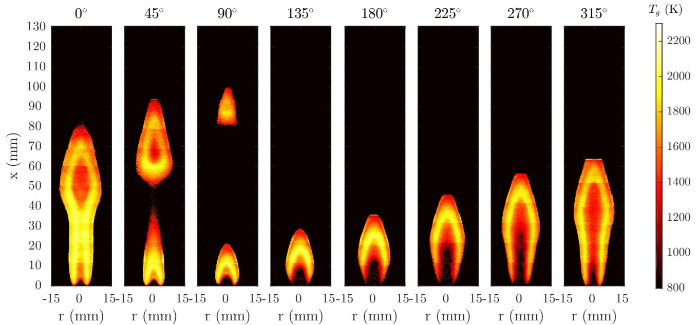
**Figure 1.18** Planar measurement of temperature,  $T_g$ , for the laminar flame with 5.6-mm-diameter burner forced at 10-Hz forcing and 50% fuel flow modulation.
