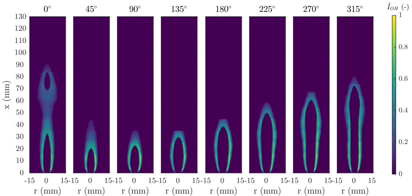
**Figure 1.11** Planar measurement of OH-LIF,  $I_{OH}$ , for the laminar flame with 4.0-mm-diameter burner forced at 10-Hz forcing and 25% fuel flow modulation.
