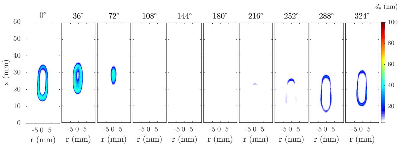
**Figure 1.6** Planar measurement of primary particle diameter,  $d_p$ , for the laminar flame with 4.0-mm-diameter burner forced at 40-Hz forcing and 50% fuel flow modulation.
