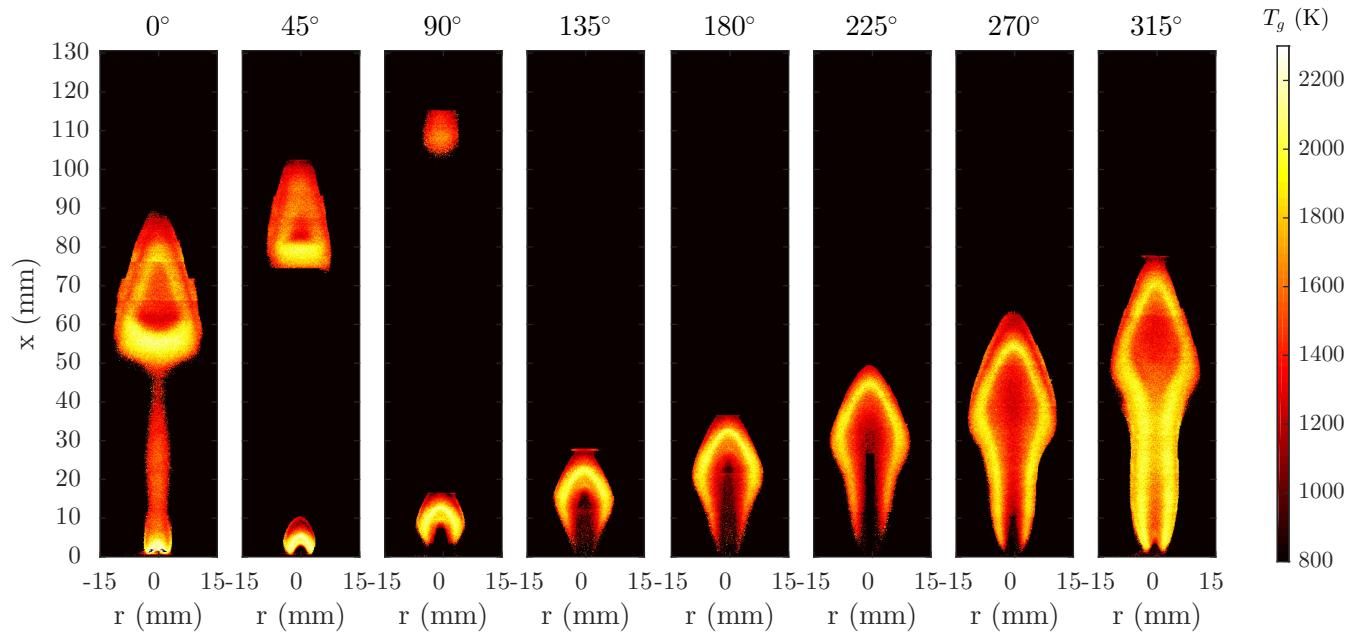
**Figure 1.14** Planar measurement of temperature,  $T_g$ , for the laminar flame with 4.0-mm-diameter burner forced at 10-Hz forcing and 50% fuel flow modulation.
