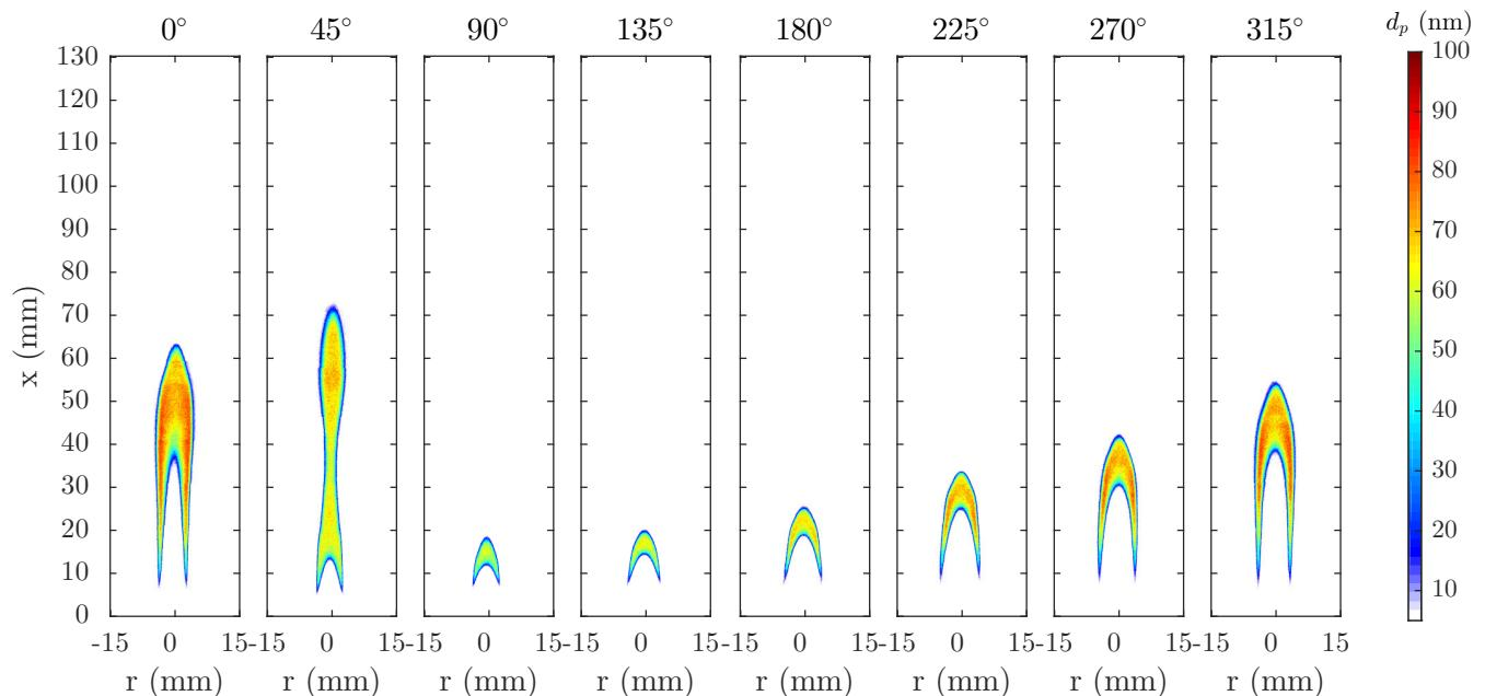
**Figure 1.25** Planar measurement of primary particle diameter,  $d_p$ , for the laminar flame with 8.0-mm-diameter burner forced at 10-Hz forcing and 25% fuel flow modulation.
