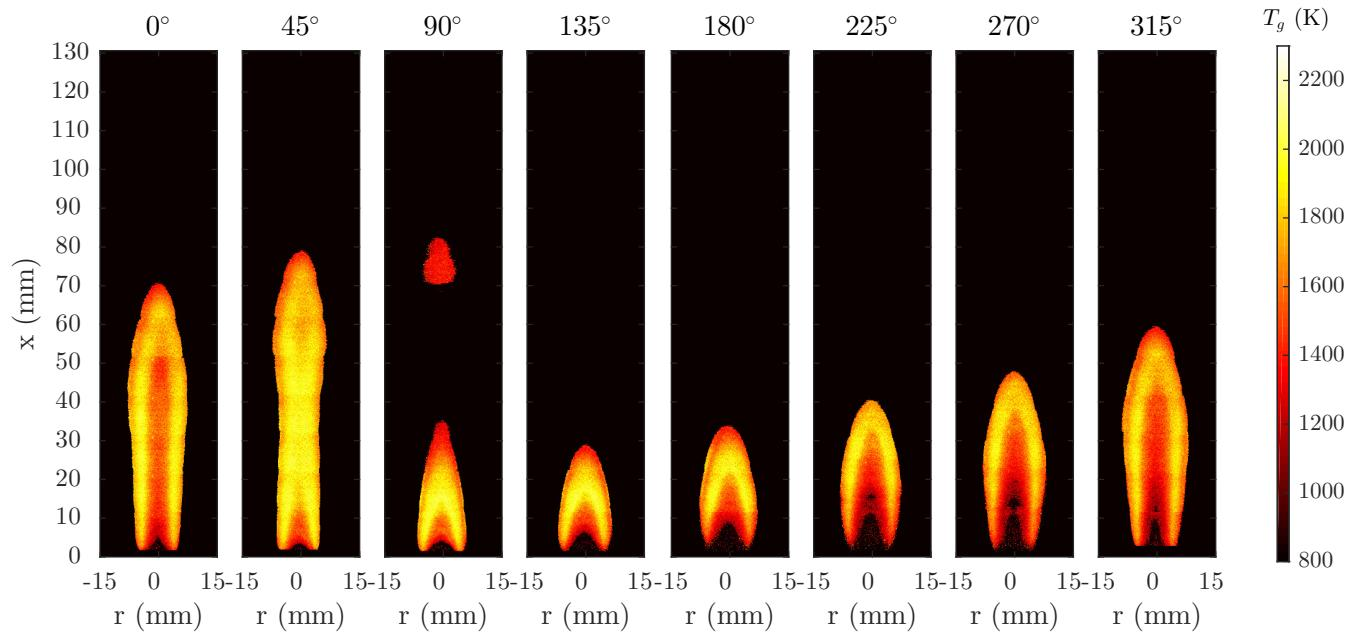
**Figure 1.26** Planar measurement of temperature,  $T_g$ , for the laminar flame with 8.0-mm-diameter burner forced at 10-Hz forcing and 25% fuel flow modulation.
