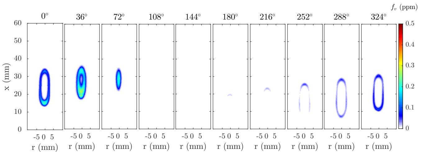
**Figure 1.5** Planar measurement of soot volume fraction,  $f_v$ , for the laminar flame with 4.0-mm-diameter burner forced at 40-Hz forcing and 50% fuel flow modulation.
