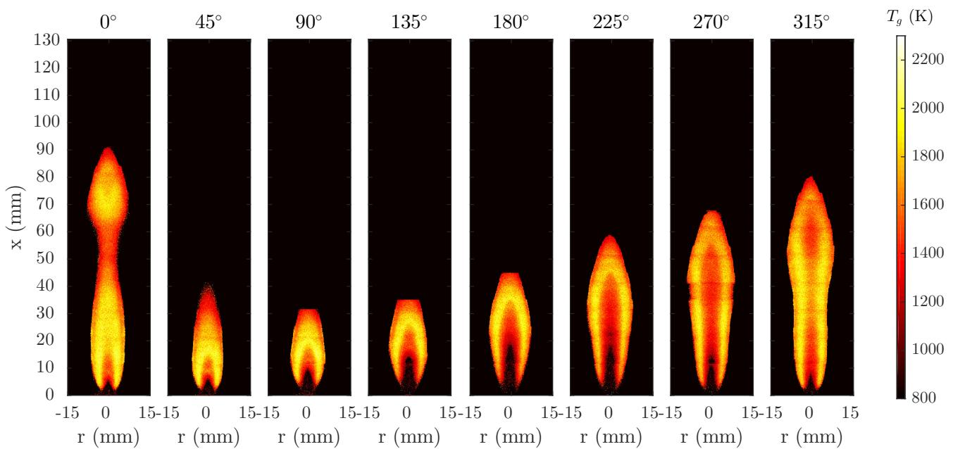
**Figure 1.10** Planar measurement of temperature,  $T_g$ , for the laminar flame with 4.0-mm-diameter burner forced at 10-Hz forcing and 25% fuel flow modulation.
