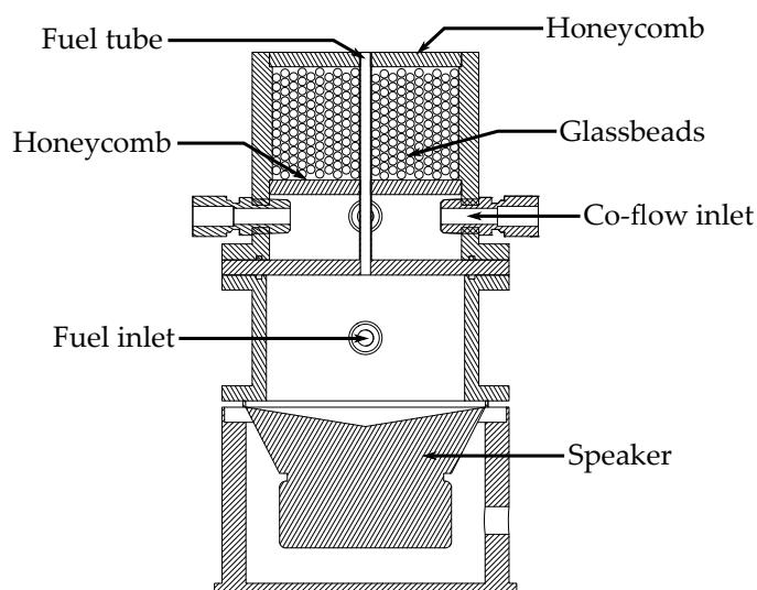
Figure 1.1 Co-flow burner for the investigation of acoustically-forced laminar non-premixed flames.
