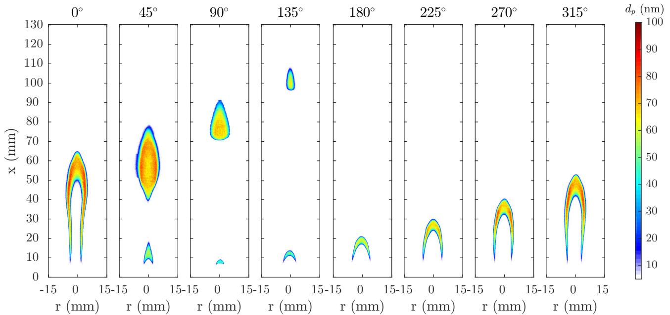
**Figure 1.29** Planar measurement of primary particle diameter,  $d_p$ , for the laminar flame with 8.0-mm-diameter burner forced at 10-Hz forcing and 50% fuel flow modulation.
