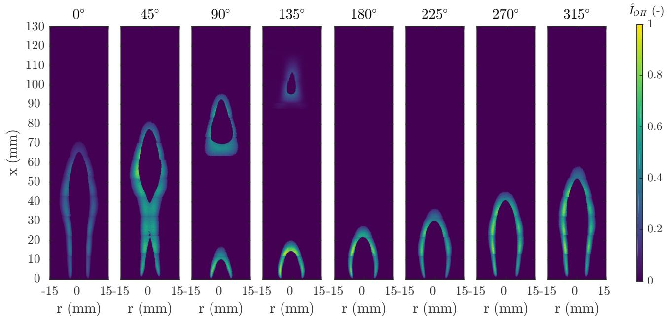
**Figure 1.31** Planar measurement of OH-LIF,  $I_{OH}$ , for the laminar flame with 8.0-mm-diameter burner forced at 10-Hz forcing and 50% fuel flow modulation.
