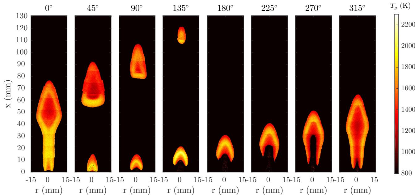
**Figure 1.22** Planar measurement of temperature,  $T_g$ , for the laminar flame with 5.6-mm-diameter burner forced at 10-Hz forcing and 75% fuel flow modulation.
