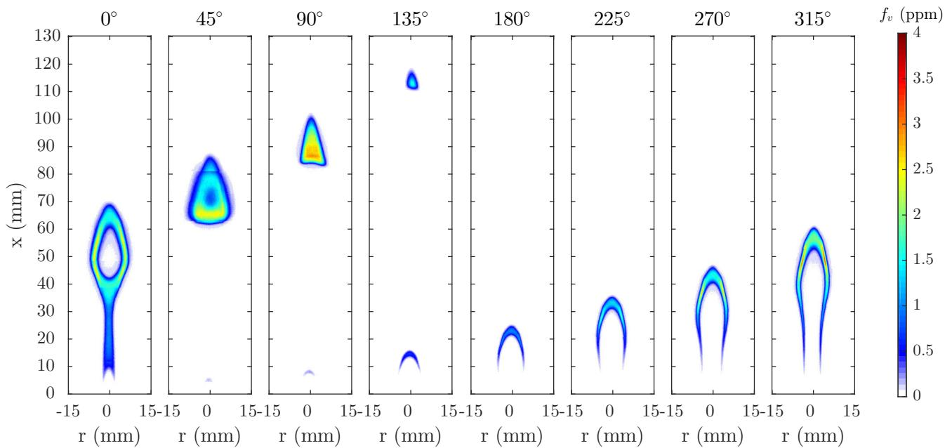
**Figure 1.20** Planar measurement of soot volume fraction,  $f_v$ , for the laminar flame with 5.6-mm-diameter burner forced at 10-Hz forcing and 75% fuel flow modulation.
