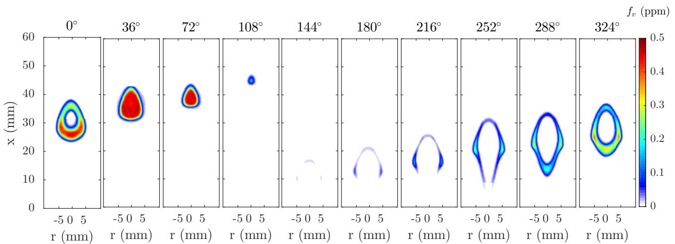
**Figure 1.2** Planar measurement of soot volume fraction,  $f_v$ , for the laminar flame with 4.0-mm-diameter burner forced at 20-Hz forcing and 50% fuel flow modulation.
