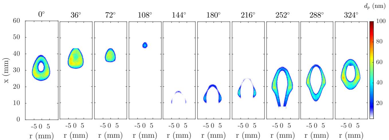
**Figure 1.3** Planar measurement of primary particle diameter,  $d_p$ , for the laminar flame with 4.0-mm-diameter burner forced at 20-Hz forcing and 50% fuel flow modulation.
