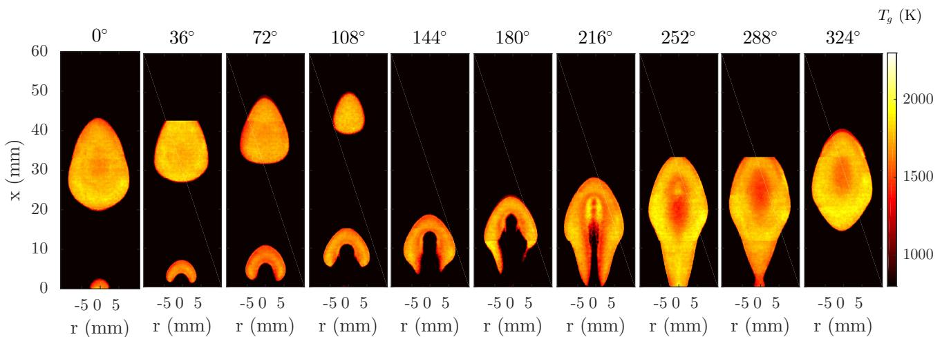
**Figure 1.4** Planar measurement of temperature,  $T_g$ , for the laminar flame with 4.0-mm-diameter burner forced at 20-Hz forcing and 50% fuel flow modulation.
