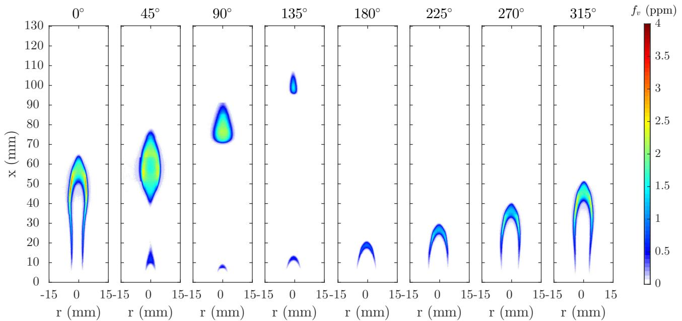
**Figure 1.28** Planar measurement of soot volume fraction,  $f_v$ , for the laminar flame with 8.0-mm-diameter burner forced at 10-Hz forcing and 50% fuel flow modulation.
