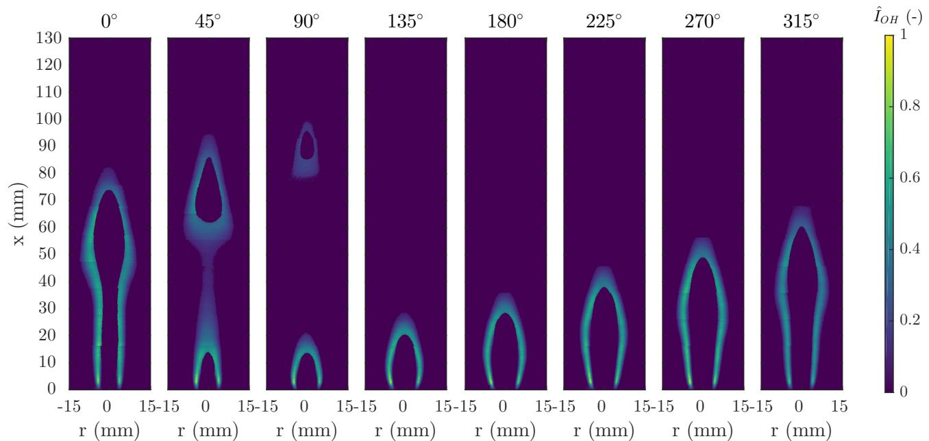
**Figure 1.23** Planar measurement of OH-LIF,  $I_{OH}$ , for the laminar flame with 5.6-mm-diameter burner forced at 10-Hz forcing and 75% fuel flow modulation.
