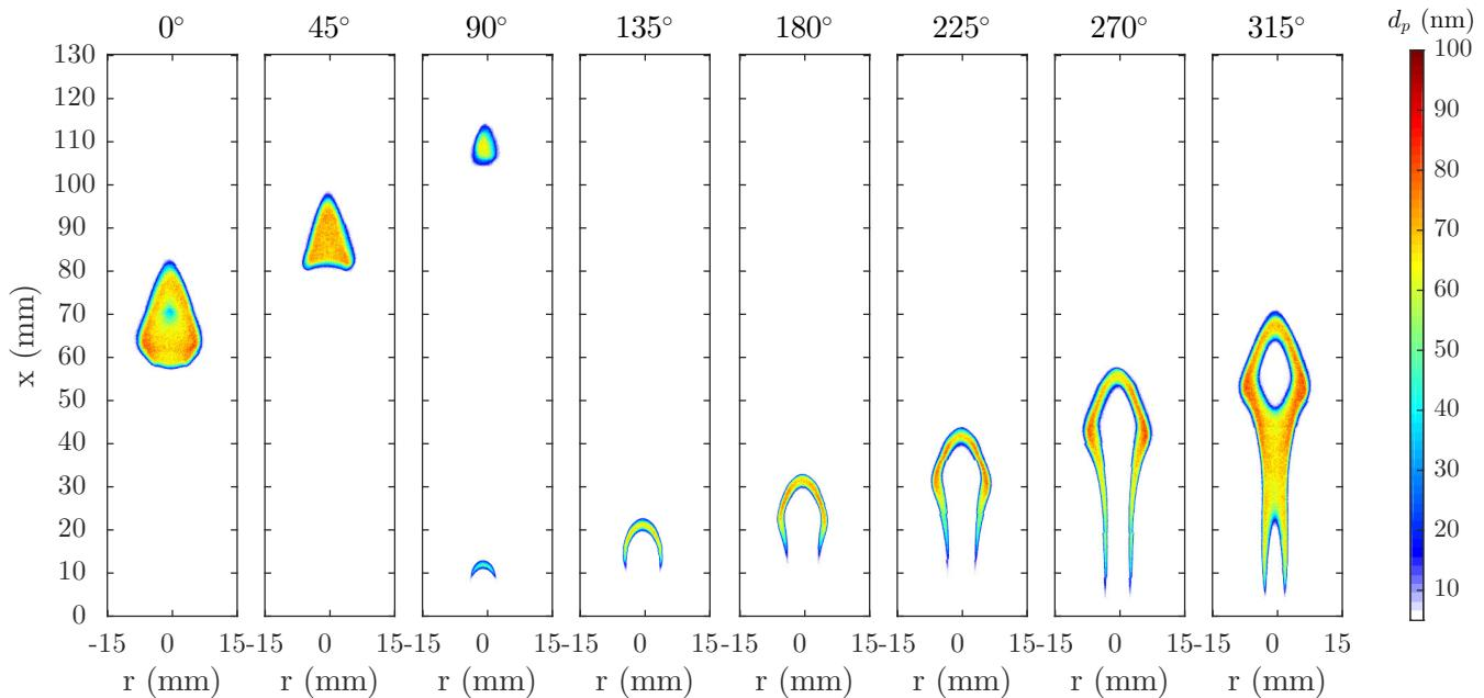
**Figure 1.13** Planar measurement of primary particle diameter,  $d_p$ , for the laminar flame with 4.0-mm-diameter burner forced at 10-Hz forcing and 50% fuel flow modulation.
