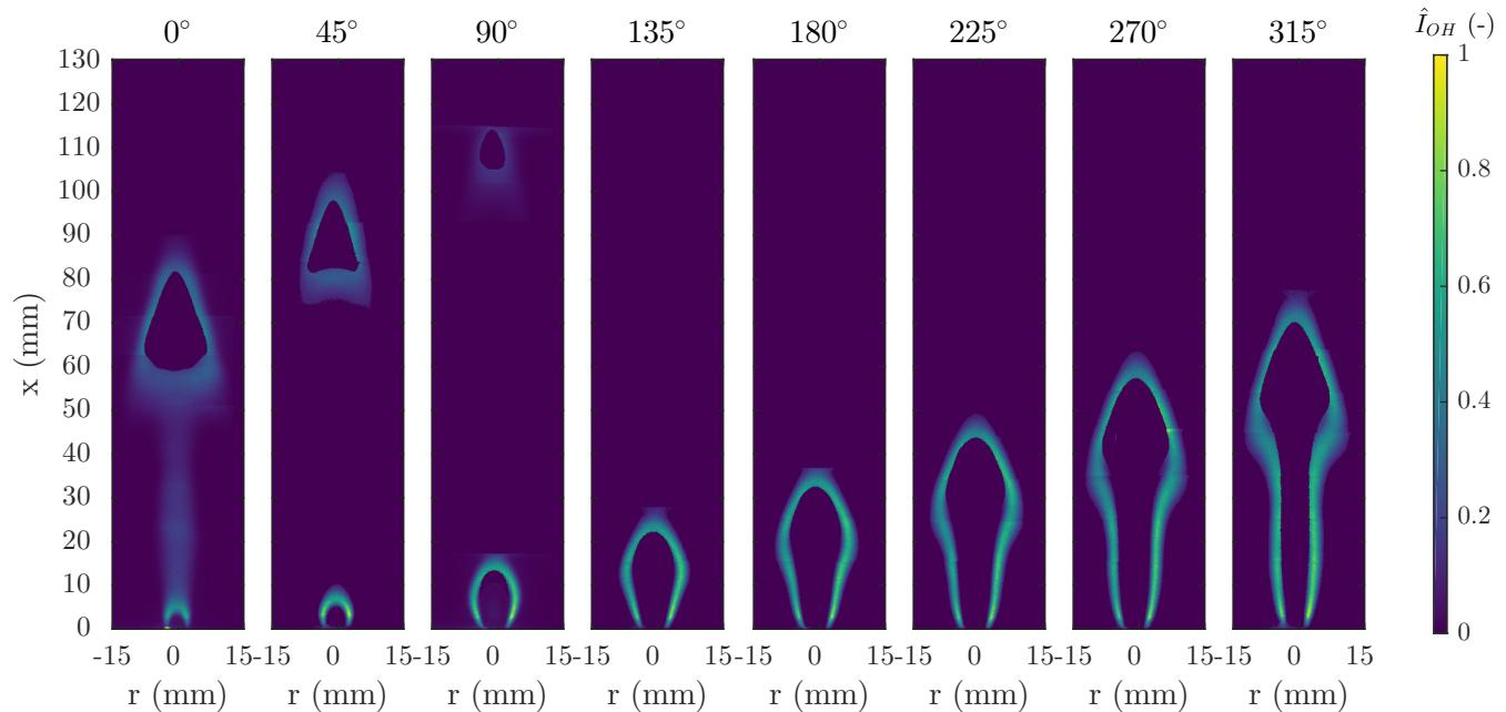
**Figure 1.15** Planar measurement of OH-LIF,  $I_{OH}$ , for the laminar flame with 4.0-mm-diameter burner forced at 10-Hz forcing and 50% fuel flow modulation.
