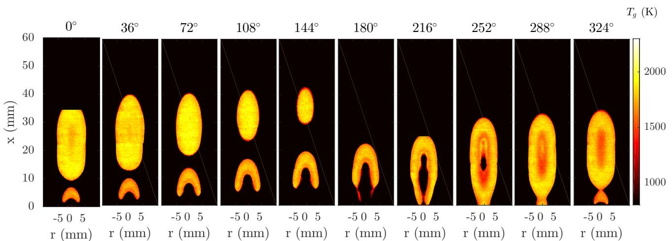
**Figure 1.7** Planar measurement of temperature,  $T_g$ , for the laminar flame with 4.0-mm-diameter burner forced at 40-Hz forcing and 50% fuel flow modulation.
