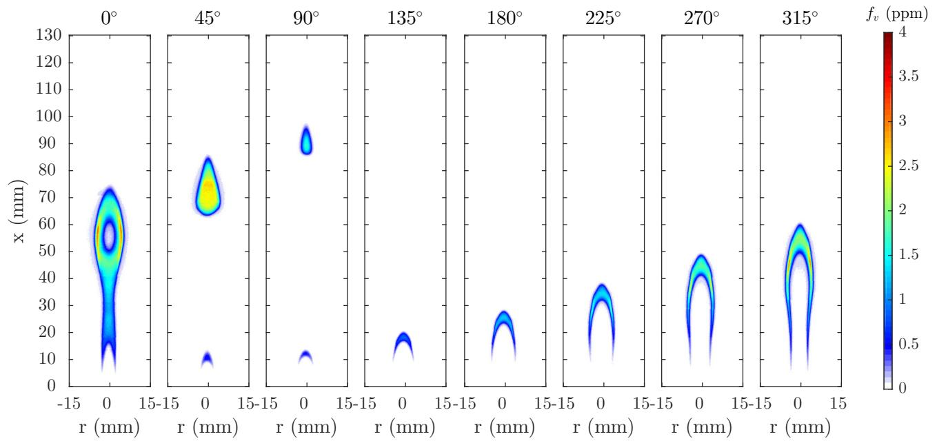
**Figure 1.16** Planar measurement of soot volume fraction,  $f_v$ , for the laminar flame with 5.6-mm-diameter burner forced at 10-Hz forcing and 50% fuel flow modulation.
