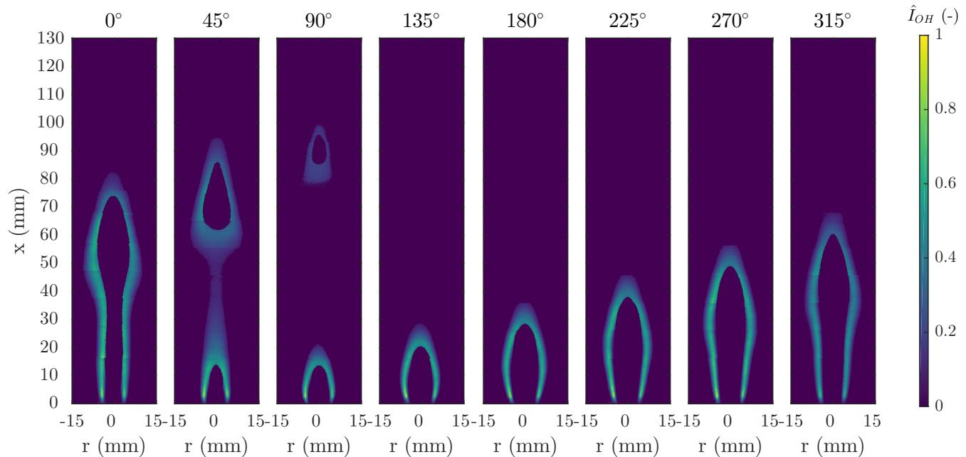
**Figure 1.19** Planar measurement of OH-LIF,  $I_{OH}$ , for the laminar flame with 5.6-mm-diameter burner forced at 10-Hz forcing and 50% fuel flow modulation.
