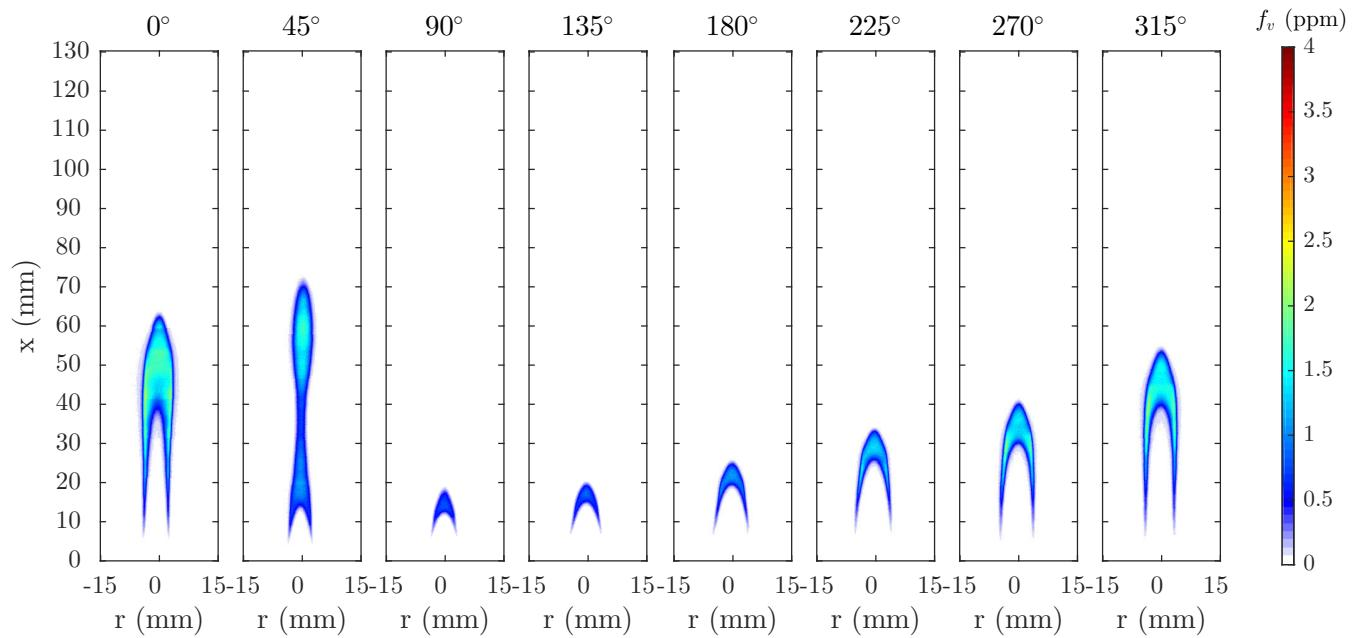
**Figure 1.24** Planar measurement of soot volume fraction,  $f_v$ , for the laminar flame with 8.0-mm-diameter burner forced at 10-Hz forcing and 25% fuel flow modulation.
