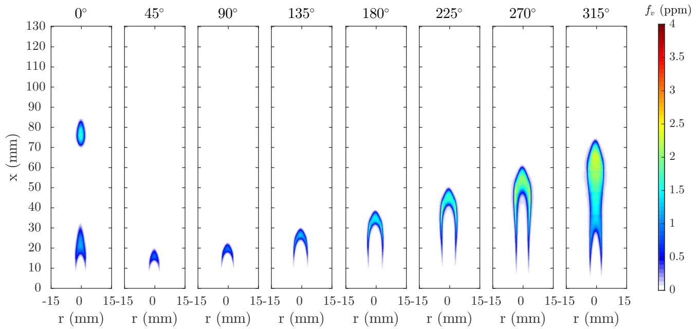
**Figure 1.8** Planar measurement of soot volume fraction,  $f_v$ , for the laminar flame with 4.0-mm-diameter burner forced at 10-Hz forcing and 25% fuel flow modulation.
