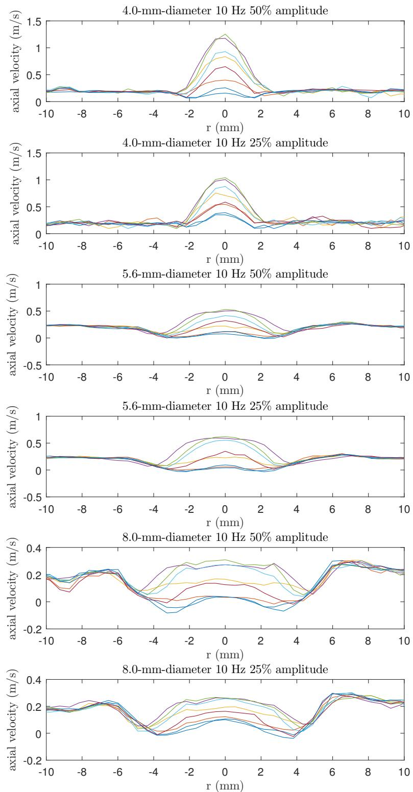
**Figure 1.32** Axial velocity profiles near the exit plane, measured in isothermal conditions using PIV.
