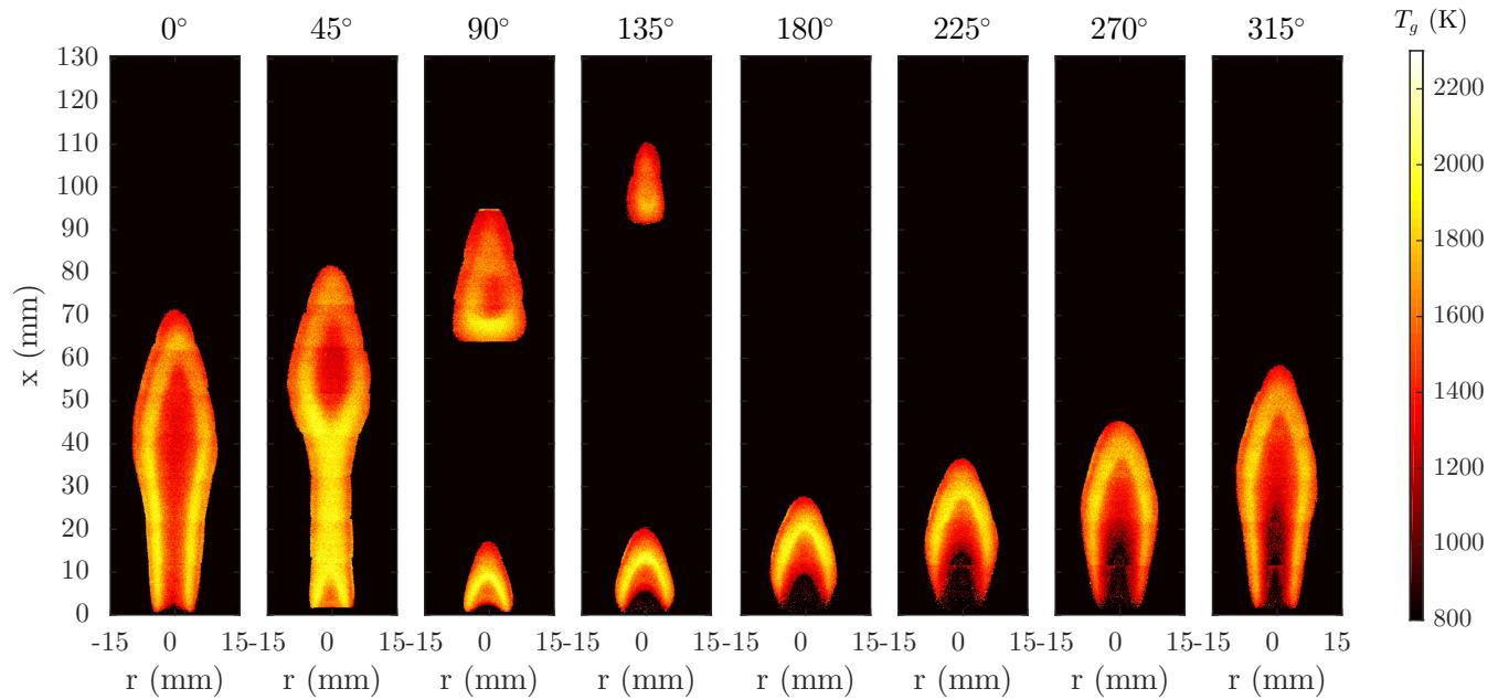
**Figure 1.30** Planar measurement of temperature,  $T_g$ , for the laminar flame with 8.0-mm-diameter burner forced at 10-Hz forcing and 50% fuel flow modulation.
