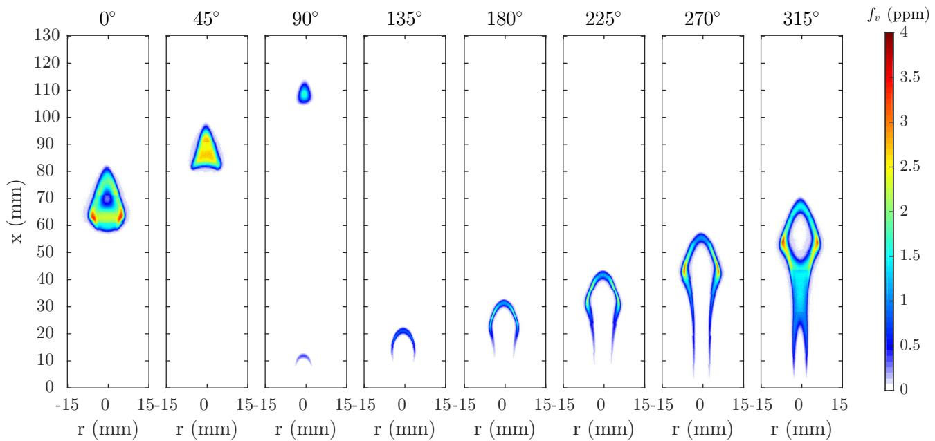
**Figure 1.12** Planar measurement of soot volume fraction,  $f_v$ , for the laminar flame with 4.0-mm-diameter burner forced at 10-Hz forcing and 50% fuel flow modulation.
