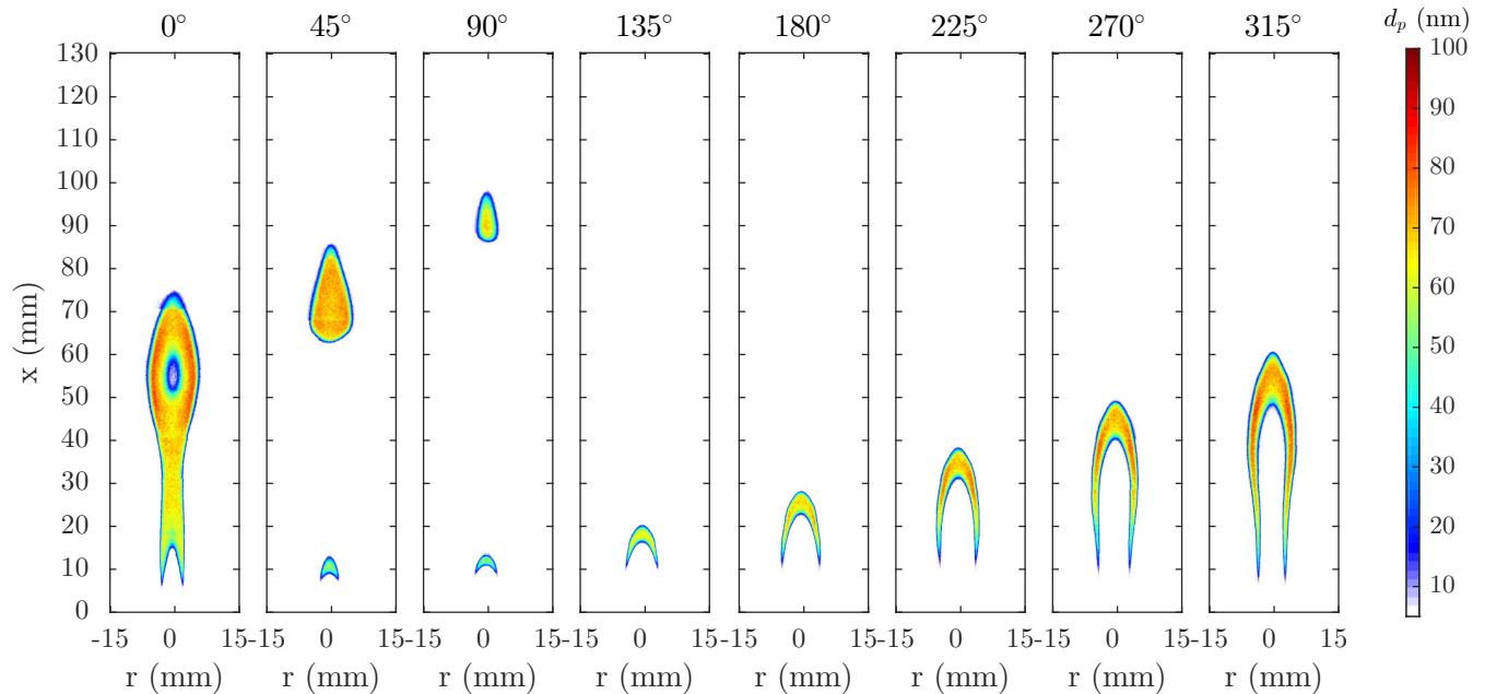
**Figure 1.17** Planar measurement of primary particle diameter,  $d_p$ , for the laminar flame with 5.6-mm-diameter burner forced at 10-Hz forcing and 50% fuel flow modulation.
