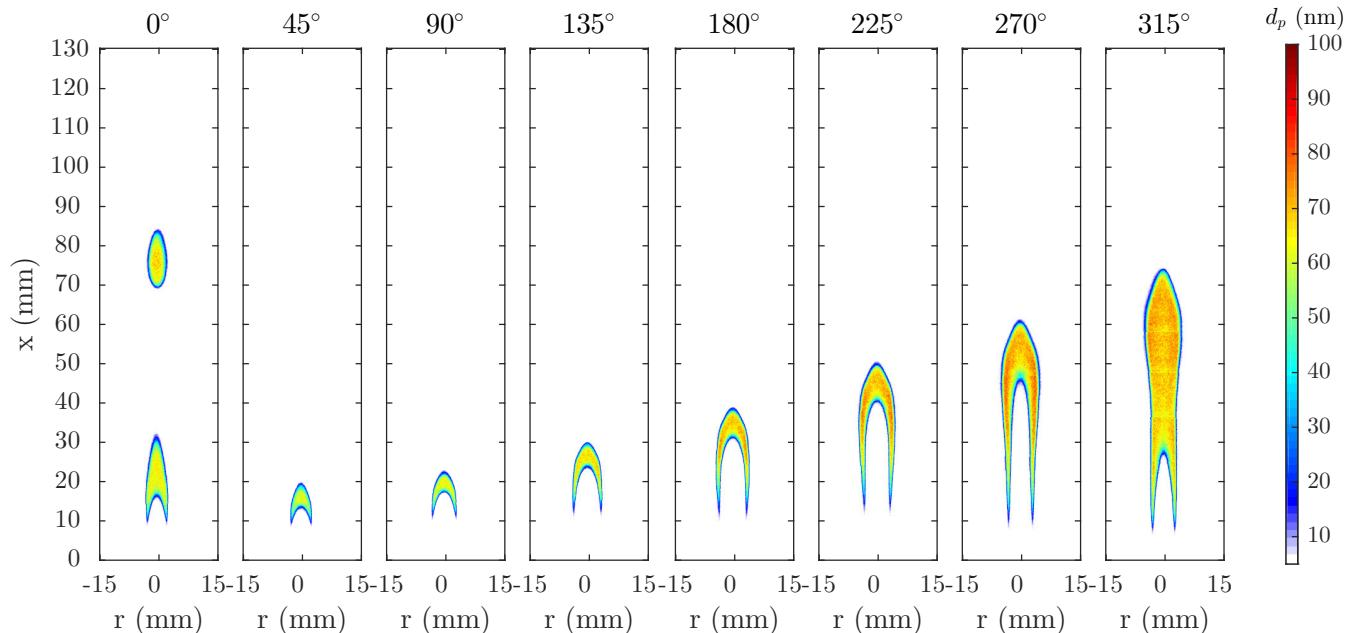
**Figure 1.9** Planar measurement of primary particle diameter,  $d_p$ , for the laminar flame with 4.0-mm-diameter burner forced at 10-Hz forcing and 25% fuel flow modulation.
