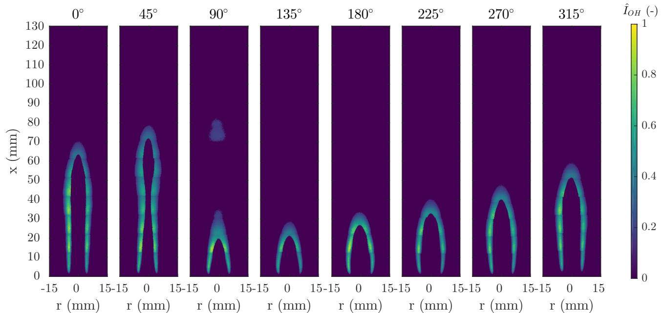
**Figure 1.27** Planar measurement of OH-LIF,  $I_{OH}$ , for the laminar flame with 8.0-mm-diameter burner forced at 10-Hz forcing and 25% fuel flow modulation.
