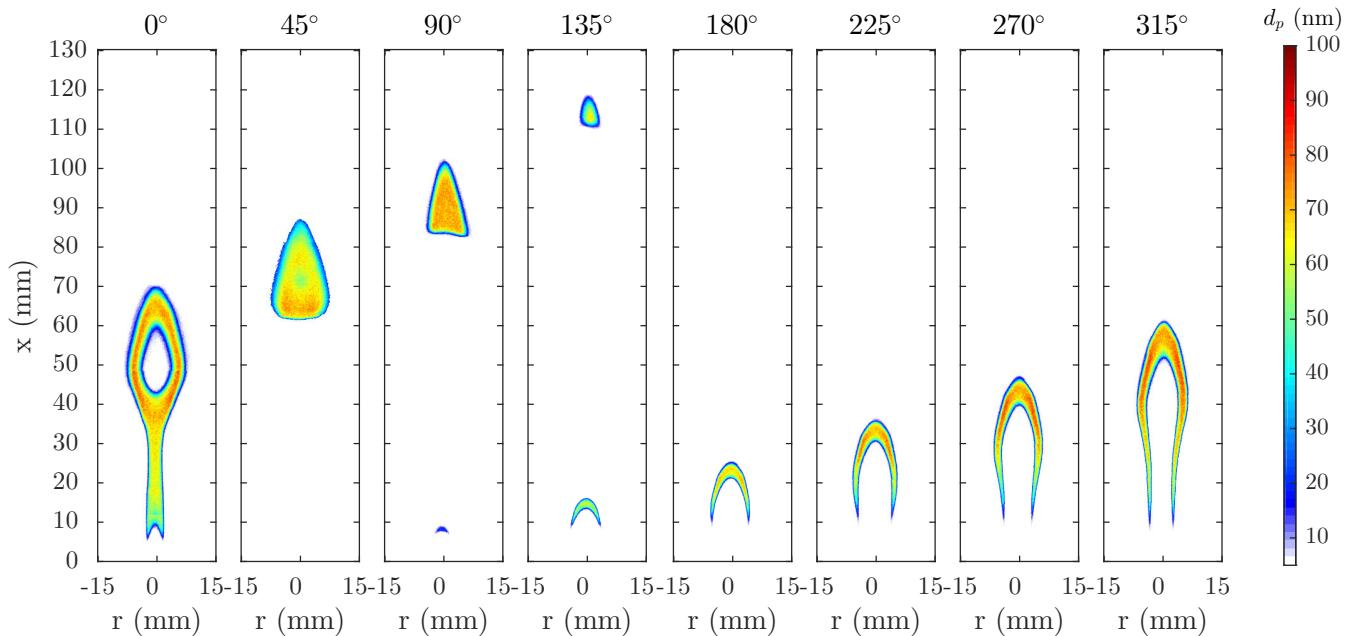
**Figure 1.21** Planar measurement of primary particle diameter,  $d_p$ , for the laminar flame with 5.6-mm-diameter burner forced at 10-Hz forcing and 75% fuel flow modulation.
