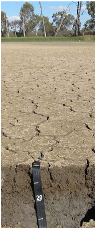
Figure 3-2 Photograph of soil profile RBAC 03 showing cracked, dark grey clay overlying a light grey heavy clay with sporadic very thin, white salt efflorescences at the surface. Hyposulfidic material occurs throughout the soil profile.
