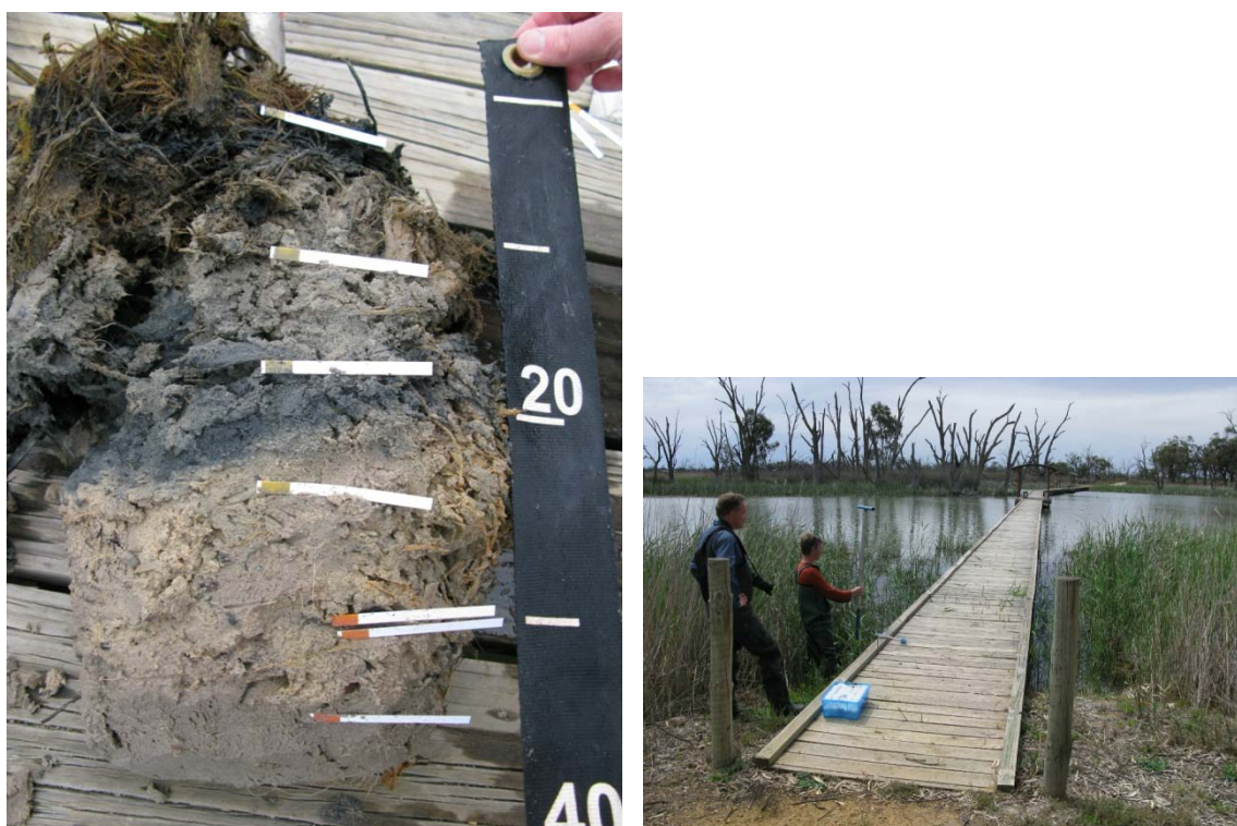
Figure 3-5 Photograph of the “Sulfuric subaqueous soil” (RBA01) profile showing sulfuric material between 25-40 cm with diffuse yellow jarosite mottles (pH <3.5: see “red” coloured pH strips indicating low pH values of 3.0) ( left hand side ) sampled under water using a shovel and placed on the boardwalk on 3 rd October 2008 when the wetland was inundated ( right hand side ).
