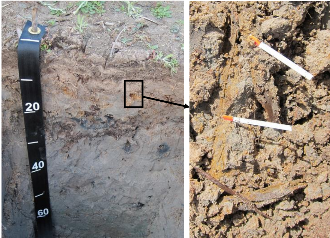
Figure 3-1 Photograph of Sulfuric soil (RBAC 01) taken on 2 nd September 2013 showing: (i) Acid Sulfate Soil with sulfuric material between 5 – 20 cm overlying hypersulfidic material (20 to 50 cm) ( left hand side ) and (ii) close-up views of the sulfuric material (pH <3.5) with bright yellow jarosite mottles (pH <3.5: see “red” coloured pH strips clearly indicating low pH values of 3.0) ( right hand side )
