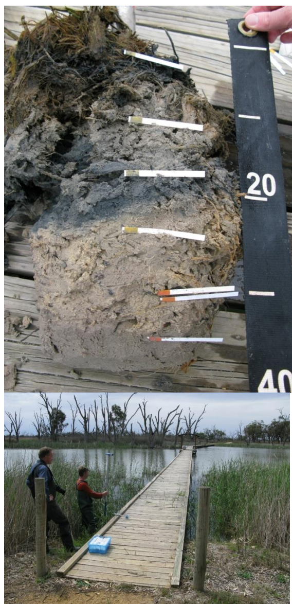
Figure 3-5 Photograph of the 'Sulfuric subaqueous soil' (RBA01) profile showing sulfuric material between 25-40 cm with diffuse yellow jarosite mottles (pH <3.5: see red coloured pH strips indicating low pH values of 3.0) ( left hand side ) sampled under water using a shovel and placed on the boardwalk on 3 rd October 2008 when the wetland was inundated ( right hand side ).
