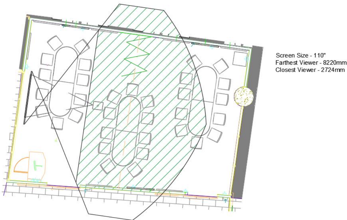
Figure 1 - Plan view showing conforming viewing area
