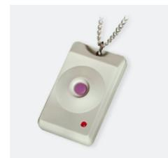
Whilst the button is pressed a red light will illuminate on the front of the pendant.
