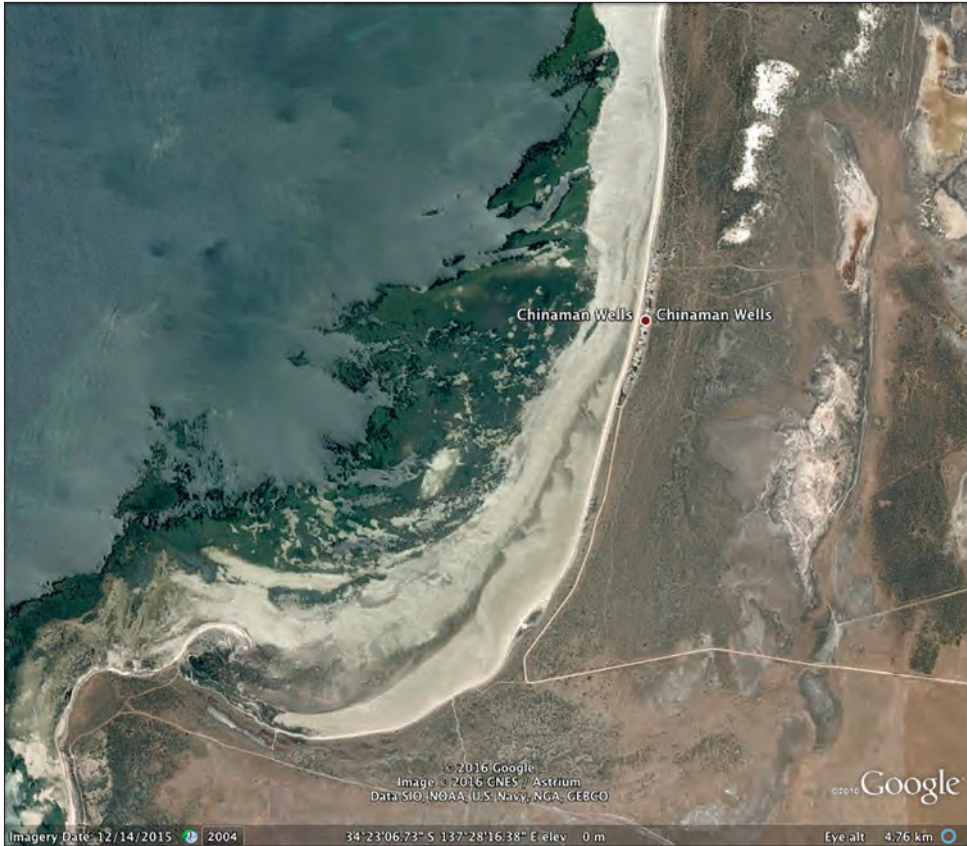
Figure 7.22 The coast at Chinaman Wells. Note the extensive intertidal platform and the broad sandy beach. Despite these features, at high tides, coastal erosion is a problem requiring rock protection for the houses.
