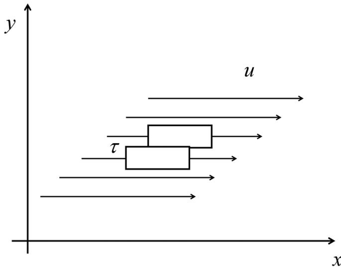
**FIGURE 8.3:** Elements of fluid slide past each other and generate a frictional shear stress.
