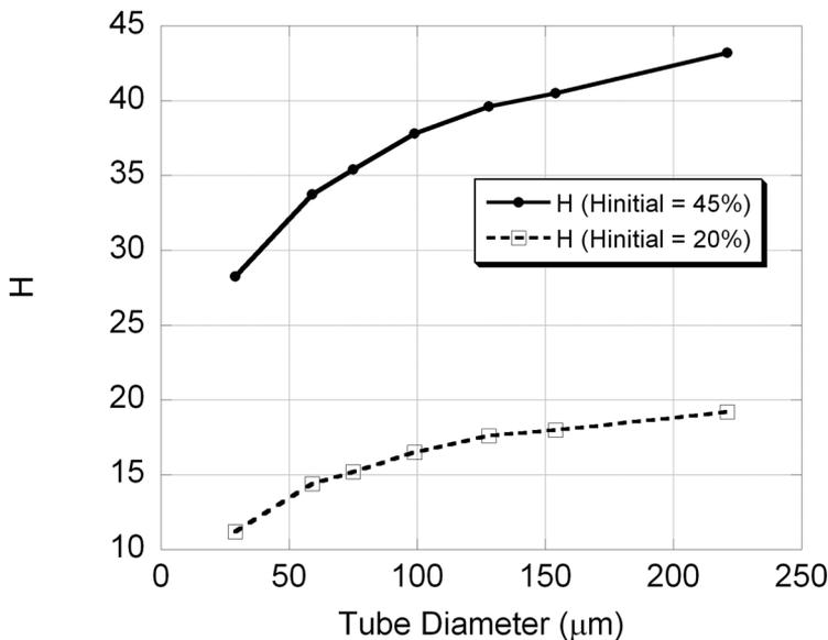
FIGURE 8.6: Hematocrit as a function of tube diameter. The initial hematocrit value for each line is shown in the inset box<sup>8</sup>.
