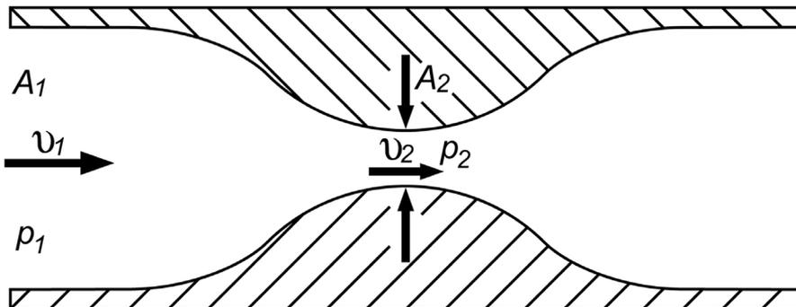
**FIGURE 8.11:** Blood vessel with a stenosis.
