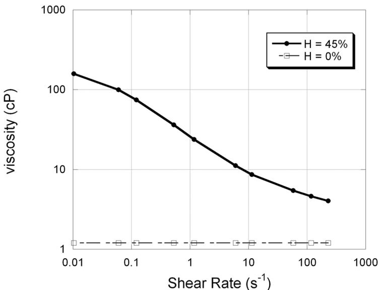
**FIGURE 8.4:** Blood viscosity as a function of shear rate for 0% and 45% hematocrit.<sup>5</sup>
