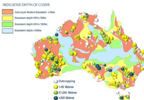
Estimated depth to basement for non-bulk mineral deposits in Australia
