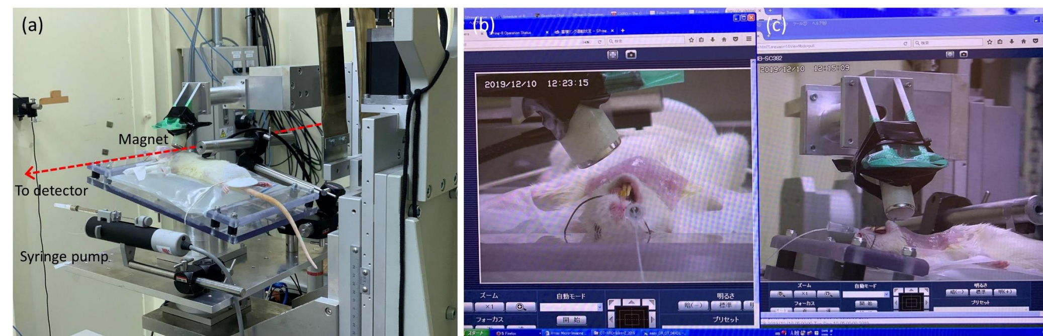
Figure 2: (a) In vivo imaging setup in the SPring-8 imaging hutch, with the path of the x-ray beam marked with a red dashed line. (b-c) The magnet positioning over the trachea was performed remotely using two orthogonally mounted IP cameras.
