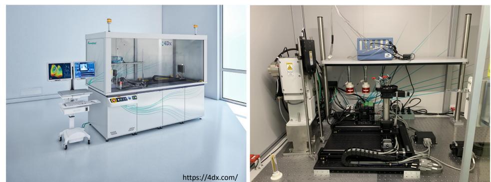
**Figure 4:** 4Dx Permetium scanner now available at the SAHMRI Gilles Plains Preclinical Imaging and Research Laboratories in Adelaide. The machine allows XV lung function studies to be performed in a range of laboratory animals including rats and mice.
