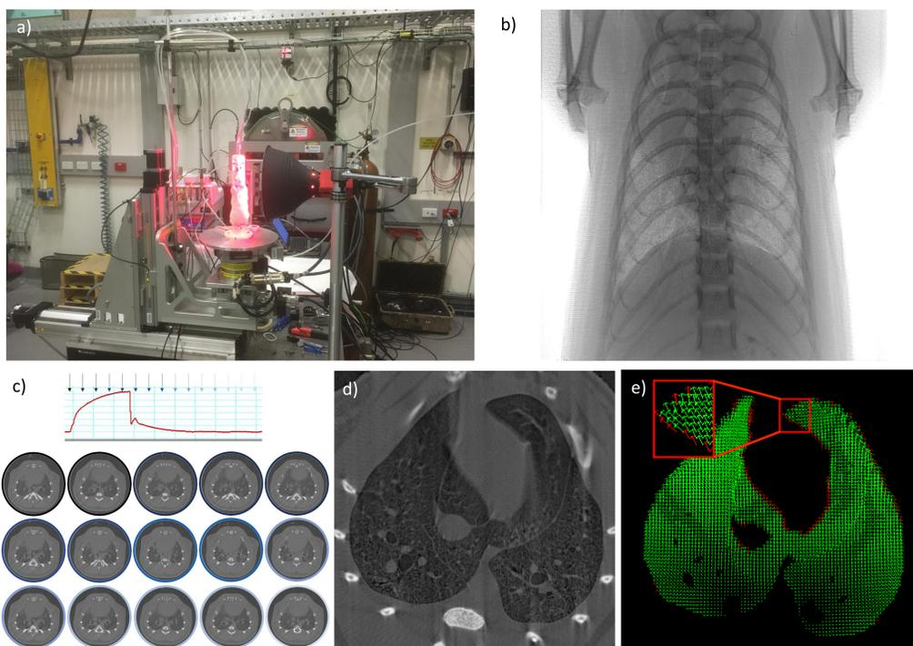
**Figure 1:** (a) The imaging setup in the IMBL hutch. (b) Example projection image. (c) Projection images are binned into the 15 phases of the breath and reconstructed. (d) Example reconstructed slice. (e) XV analysis produces a vector map that shows how the lung tissue moves during the breath (green indicates a confident measurement, red indicates some uncertainty).
