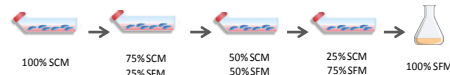
Figure 1: Sequential process of adapting adherent HEK 293FT cells in DMEM/10%FCS to FreeStyle™ serum-free media in suspension culture. SCM = serum-containing media, SFM = serum-free media [2].
