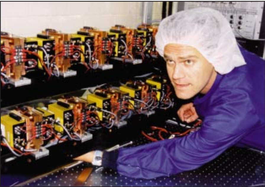
Dr Martin Ostermeyer, a Feodor Lynen Fellow from Germany and a member of the research team, installs infra-red diode-lasers to provide the energy source for the stable laser. Photo: Rob Morrison.
