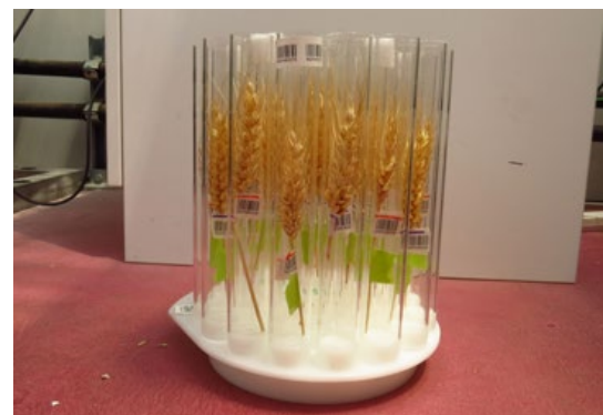
Grain in cassette to be deployed in our new GRDC funded X-Ray CT Scanner - Plant Accelerator
